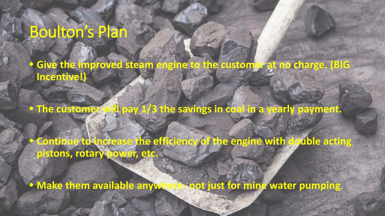
Boulton & Watt Steam Engine-Rotary Power
